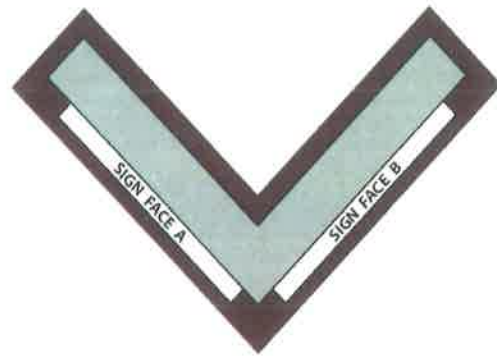
TOP VIEW OF "V"-SHAPED FREESTANDING SIGN
